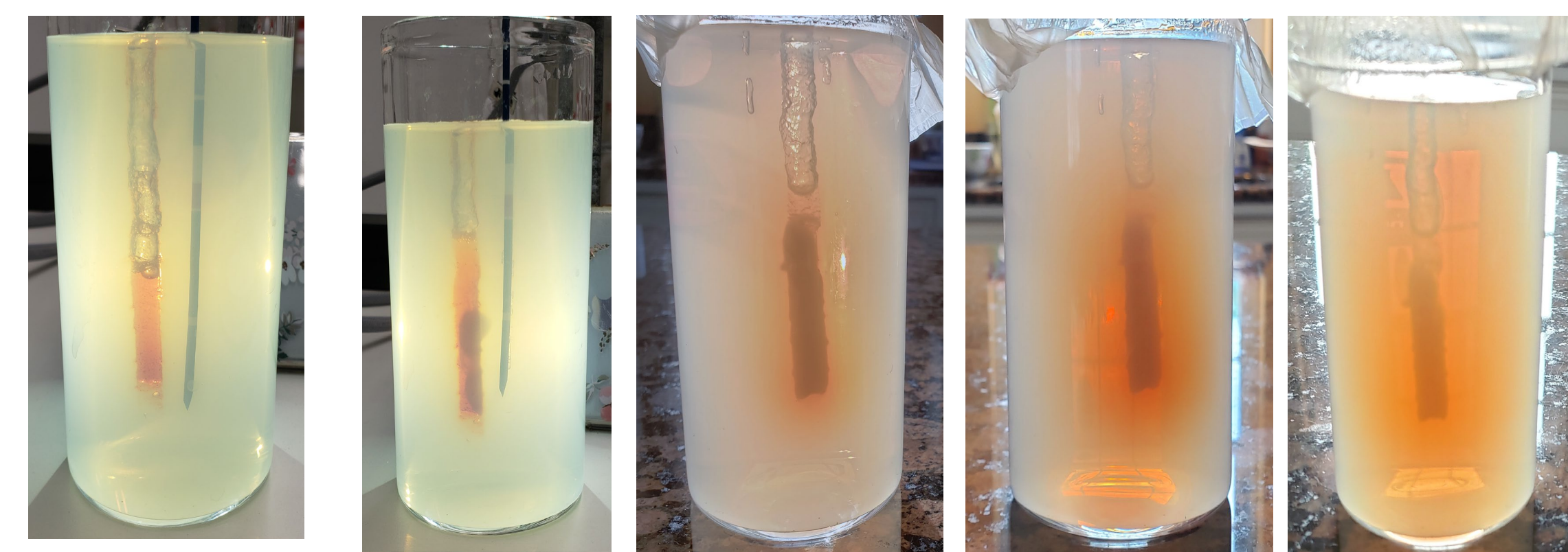
Figure 2. The drug elution of Doxorubicin+HeatSYNC Gel, before ablation (far left), during ablation (3 min), 6 h, 24h and 48h post ablation, respectively. 1 %(w/v) agarose phantom. The ablation conditions: 915 MHz, 60W for 10 minutes.
