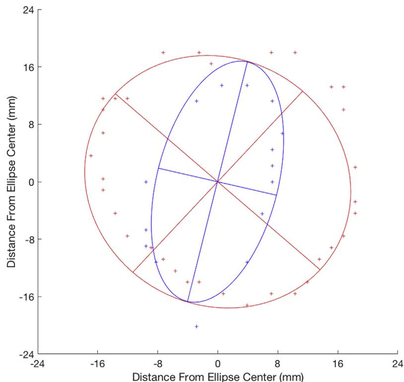
**Figure 5.** Thermal energy eccentricity of representative MW ablations performed without (blue) and with (red) thermal accelerant in the same animal. When the accelerant gel was administered, the volume of thermal energy within the ablation zone was significantly larger and more spherical in shape. Hash marks correspond to outer ablation zone boundaries, defined according to a temperature threshold of  $60^{\circ}\text{C}$ .
